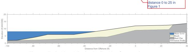
Figure 1. Typical Beach Design Profile, After Construction
