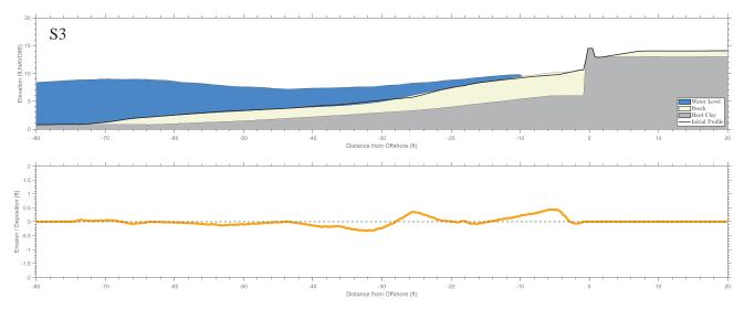
Figure 12. Seawall-Beach Profile Response Under Storm Wave Conditions and MHW Tide.
