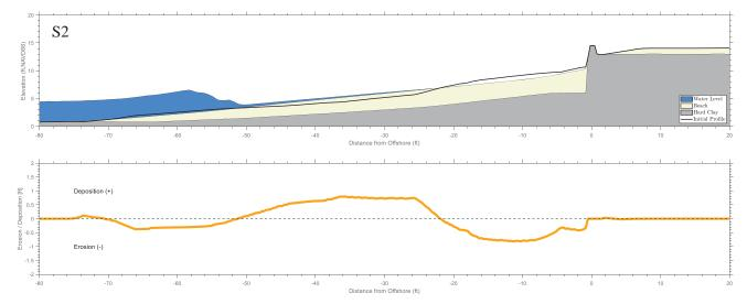
Figure 11. Seawall-Beach Profile Response Under Storm Wave Conditions and Full Tide Range.
