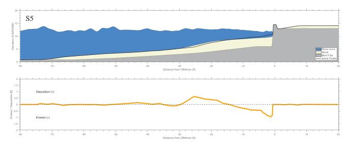
Figure 14. Seawall-Beach Profile Response Under Storm Wave Conditions and 100-Year SWL Event
