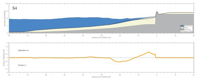
Figure 13. Seawall-Beach Profile Response Under Storm Wave Conditions and 1-Year SWL Event.
