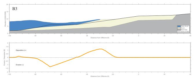
Figure 8. Beach Profile Response Under Storm Wave Conditions and MHW Tide.
